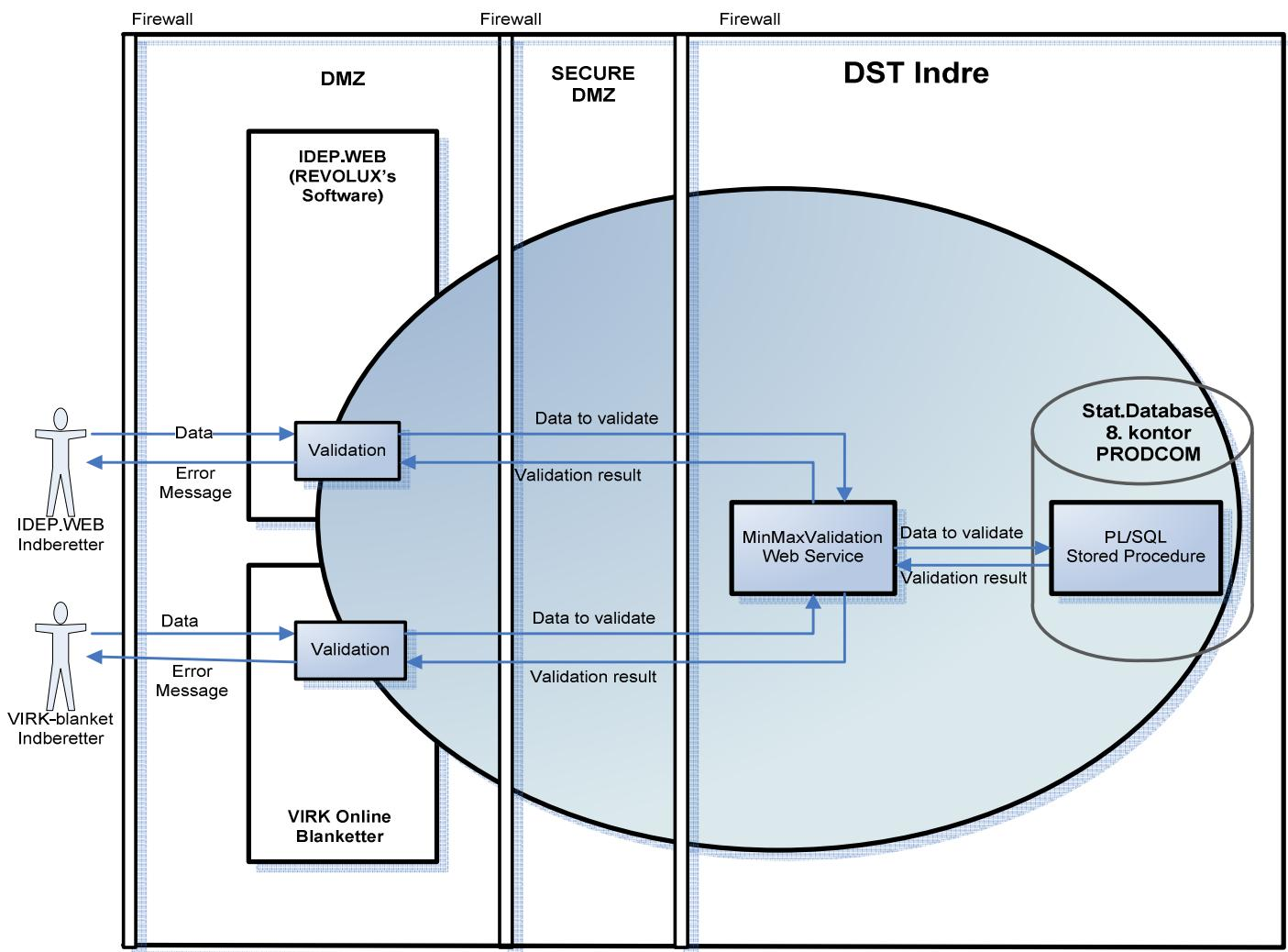
With respect to data security, there is no direct connection between the User Interface and the statistical database. The connection must go via Web Service (MinMaxValidation) and through firewalls and Secure Zone.
